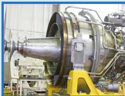
GTD-10RM engine for the automatic gas-pumping unit GPA-10RM
