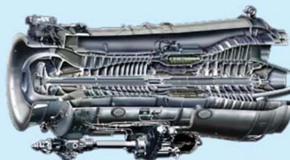
Power-driven gas-turbine engine, 6, 8 MW
