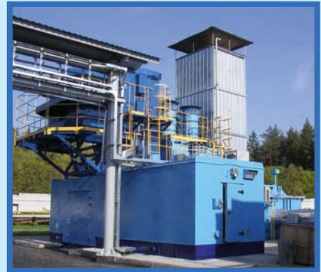
Gas-pumping unit with the capacity of 6,3 MW
