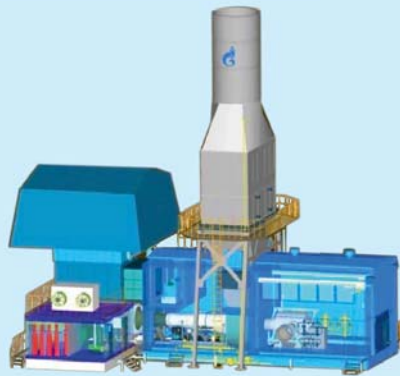
Gas-turbine unit with the capacity of 16 MW
