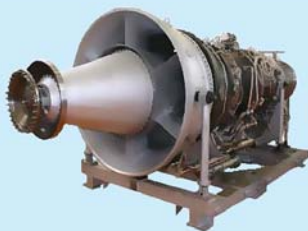
Mechanical gas-turbine engine with the capacity of 16 MW
