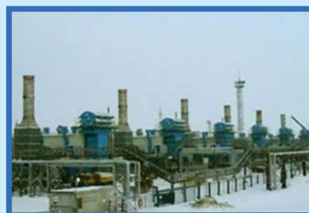
Booster gas-pumping unit with the capacity of 16 MW at the compressor station of Yamburggazdobycha Production Association
