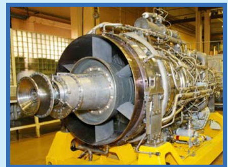
GTD-6,3RM engine for the automatic gas-pumping unit GPA-6,3RM
