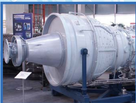
AL-31ST engine for gas-pumping Units with the capacity of 16 MW
