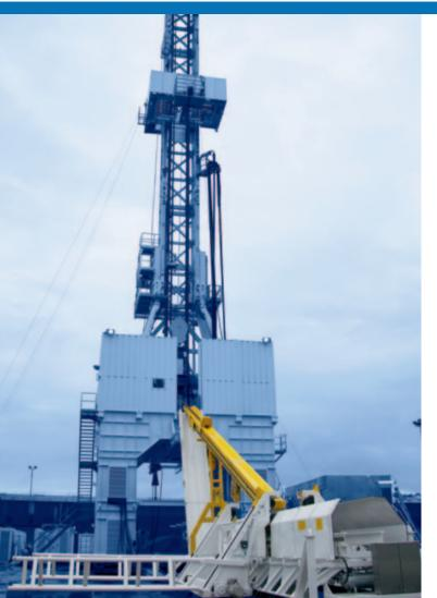
The Bentec MECHANIZED CATWALK SYSTEM (MCS) simplifies and speeds up pipe handling from the pipe rack to the drill floor. By lifting the pipes to the drill floor, they can be directly picked up by an elevator, sparing the need for time-consuming interim storage in the mouse hole.
