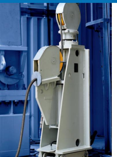
This useful rig floor equipment provides smooth, adjustable make-up loads. Due to its hydraulic operation, the Bentec Cathead eliminates electrical hazards. The system can be powered by an independent hydraulic power unit (HPU) or integrated into a centralized hydraulic unit (CHPU).
