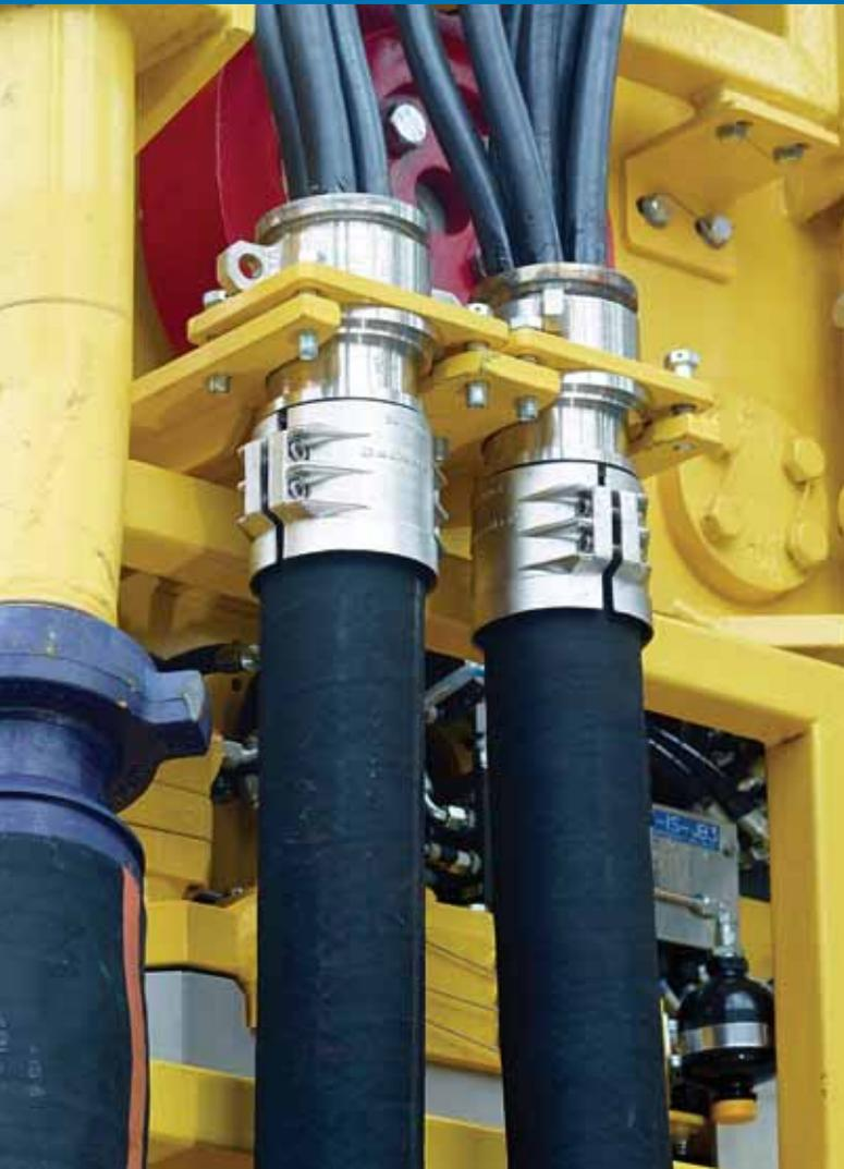
Bentec SERVICE LOOPS provide a highly reliable power and control supply solution for all common Top Drives and are interchangeable with the OEM service loops. By casting the power plugs and the end of the outer tubes, Bentec SERVICE LOOPS are able to withstand harsh environments and highest mechanical tractive forces.
